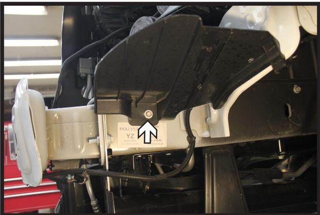
11. On the driver side, using a 10MM socket, remove the screw from the plastic shield. The shield will not be reinstalled.
