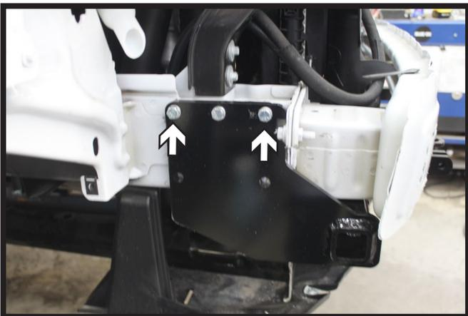
15. Continue drilling the remaining top holes thru the frame with a 3/8" drill bit. Installing 3/8" bolts with lock washers into the holes with a 3/8" whiz nuts on the inside of the frame lip. Do this on both sides of the vehicle. Fully tighten the all hardware.
