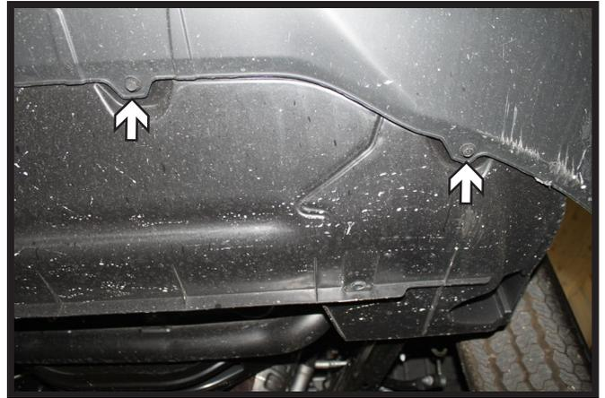
6. Using a 10MM socket, remove the four (4) screws from the underside of the fascia. There are two (2) on each side.
