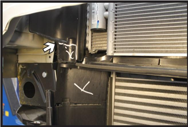
13. Trim the upper section of shielding just below the bumper and disconnect the lower section. Do this on both sides of the vehicle.
