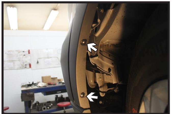
4. Remove the two (2) push pins from along the edge of the wheel well. Do this on both sides of the vehicle.
