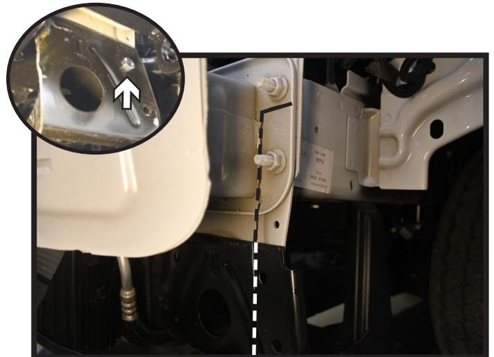
12. Using a reciprocating saw, trim off the frame flange just below the top bolt back to the face of the frame and all the way down. Do this on both sides of the vehicle. Install the supplied 3/8" bolt and lock nut into the upper inner existing hole where the crossbar attached (inset) and fully tighten.
