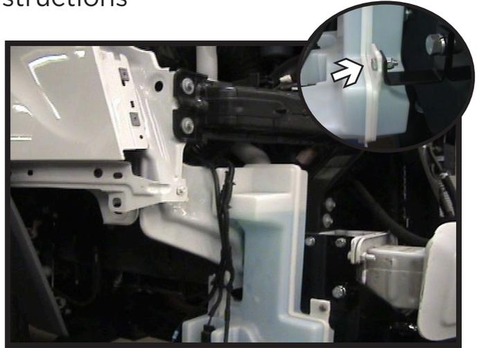
18. Reinstall the washer reservoir onto the vehicle. Use the supplied 1/4" hardware to attach the reservoir to the bracket as shown.
