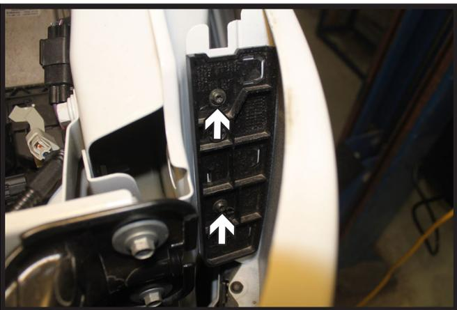
3. Underneath where the headlight was, using a T25 Torx, remove the two (2) screws from the fascia/fender joint. Do this on both sides of the vehicle.
