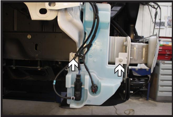
9. Using a 10MM socket, remove the two (2) screws from the washer reservoir. Disconnect/plug all lines and set the reservoir aside.
