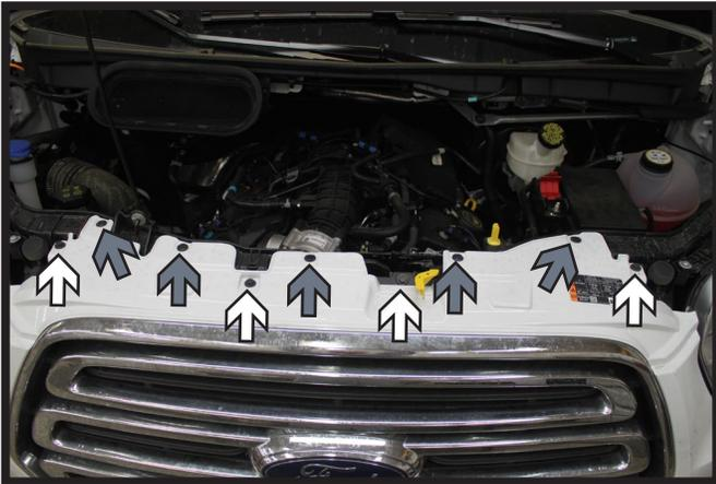
1. Using a 10MM socket, remove the four (4) screws from the top edge of the fascia (white). Then remove the five (5) push pins (gray).
