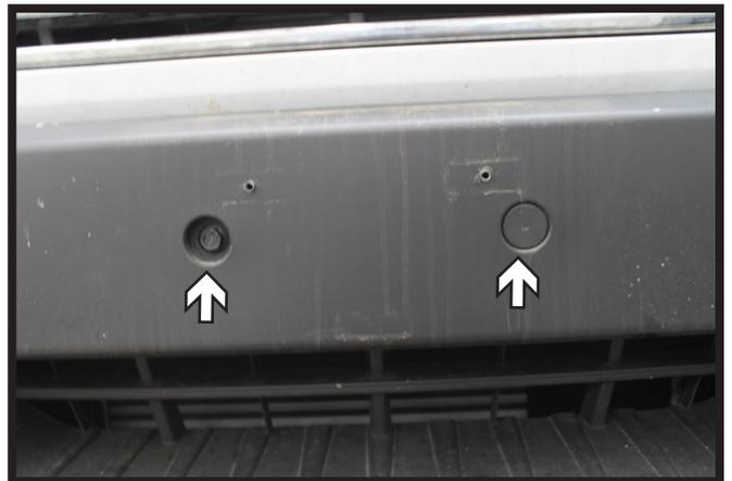
8. Remove the plugs from the fascia. Then using a 13MM socket remove the two (2) screws from the face of the fascia. Pull the corners of the fascia away from the vehicle disconnecting any electrical connections and set the fascia aside.
