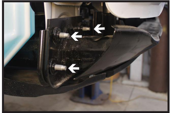
10. Using a 13MM socket, remove the four (4) bolts from the backside of the crossbar. Do this on both sides of the vehicle. The crossbar will not be reinstalled.
